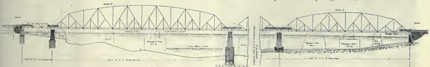
Fig. 1.—Part of side elevation Moncton Bridge showing end span—3 centre spans similar to span A not shown—Total length of bridge 1787 ft. Note relative size of present and new piers.
